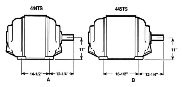
The length difference in the examples above occurs between the feet as shown by dimensions A and B. The suffix T indicates that the motor frame assignment conforms to the current, or so called "T" frame "Nu-Rate" standards which were adopted in 1964.
